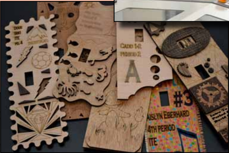
Locker Tags designed using CADD software and then imported into the Laser Cutter program for cutting and scanning. The designs were created by the students and the tags will be used to claim lockers to store materials in the STEAM lab when working on projects.
